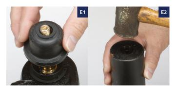
Install the grease fitting and properly grease the part per the instruction sheet (if applicable).
