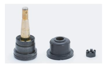
After installing the ball joint into the control arm or steering knuckle, follow the suggestions below to install a press-fit style MOOG boot. It is important to install the MOOG boot properly to prevent damage to the boot and to prevent excessive grease from squeezing out onto brake components when lubricating.
